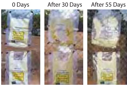
Illustration of photo and thermal degradation of a carrier bag incorporating EPI's Oxo-Biodegradable technology (top row) vs. a bag without EPI's Technology (bottom row). Test procedures follow ASTM D5272 "Outdoor Exposure Testing of Photo Degradable Plastics" Guidelines.
